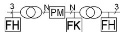
Fig. 1. Block diagram of phase shifter with matrix converter (PM); FK – switching filter, FH – harmonic filter
