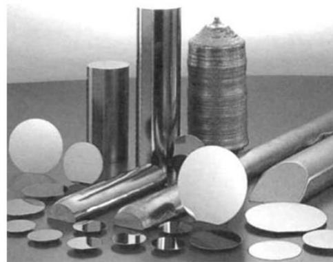
**Figure .1: Compound semiconductors such as GaAs and InP**
